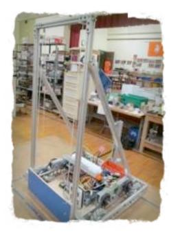
robot, Metal Arc, to tip the teeter-totter ramp.
